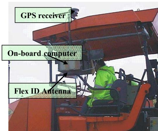
Figure 4: The paver on-board computer and GPS antenna
