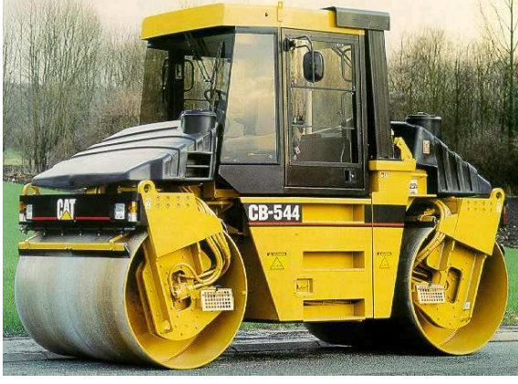
Fig. 1. A typical compactor: Caterpillar CB544
