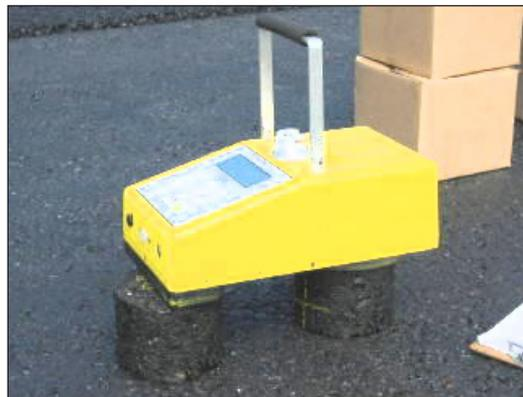
This Troxler PaveTracker, shown here testing asphalt specimens produced by a Superpave Gyrotory Compactor, will be easier and safer to use in quality control of HMA density than nuclear density gauges (Fig. A.4 of the final report).
