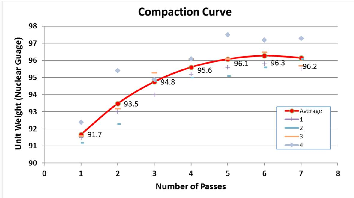
**Figure 72: Compaction Curve from the Trial Section on 10/21/2016 (Project No. 6 - J2P3051, RT 24).**
