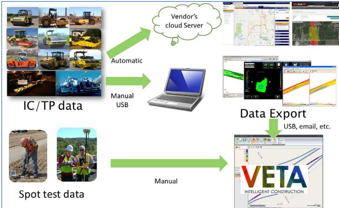
**Figure 8. IC and IR Data Flow to Veta.**
