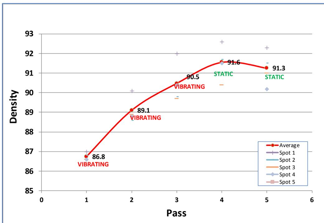
Figure 39: Compaction Curve from the Trial Section on 4/24/2017 (J1P3005 RT 24).
