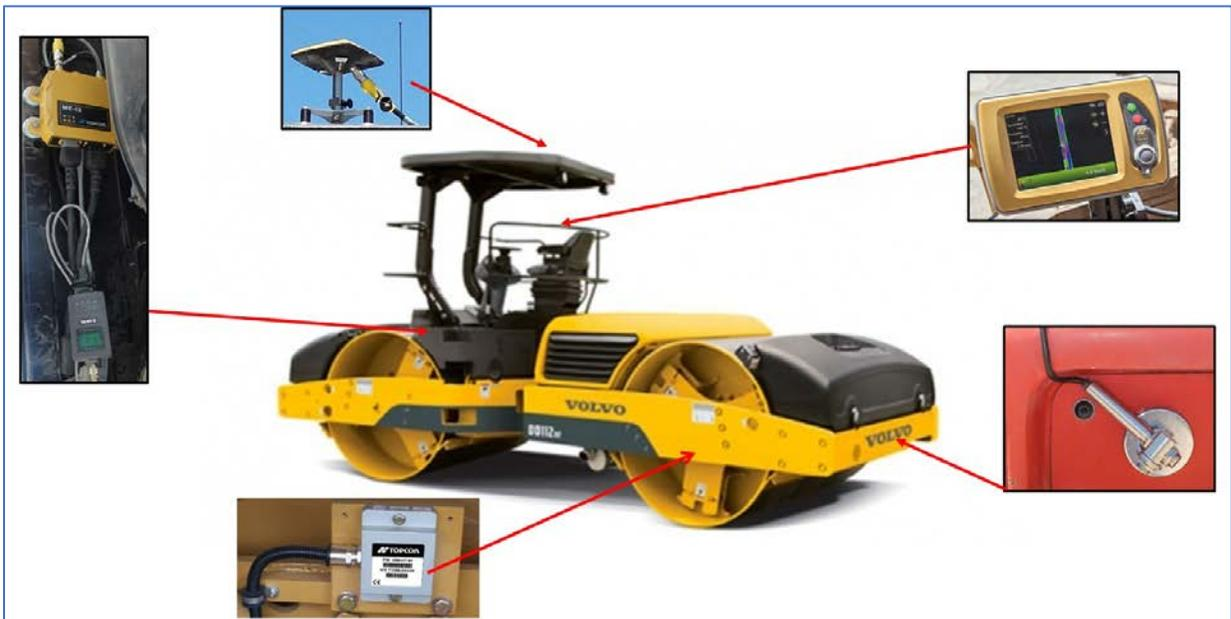
**Figure 3. An Example of IC Retrofit Systems.**
