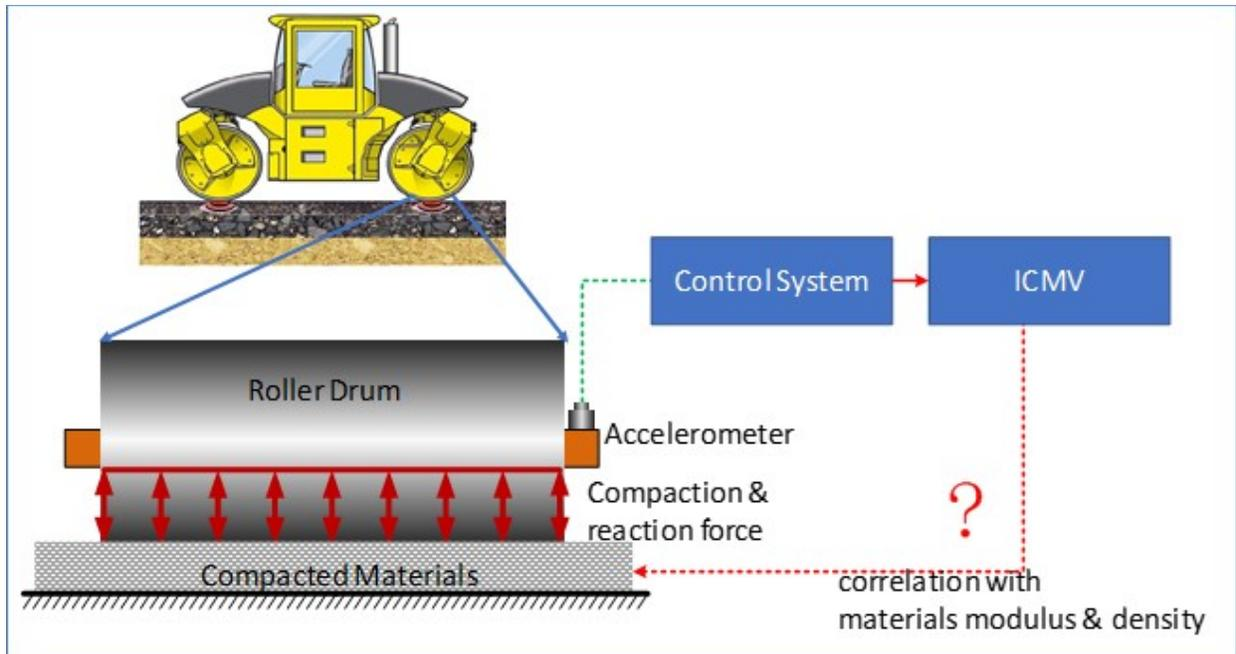
**Figure 4. Method of Measuring and Calculating ICMV.**
