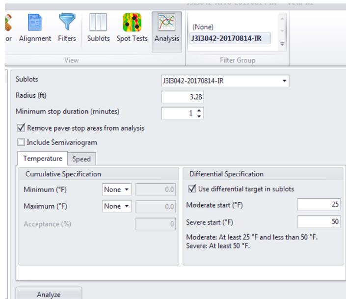
**Figure 29: Example of a Veta Analysis setup for IR data analysis (J3I3042, RT70).**
