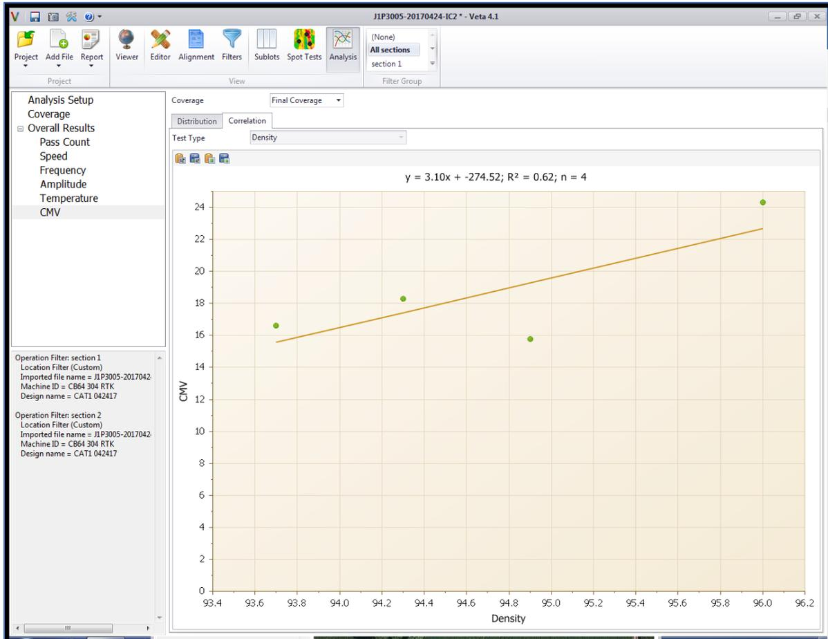
**Figure 43: An Example Veta Analysis Screen showing correlation tests between ICMV and spot tests (JIP3005 RT 24).**
