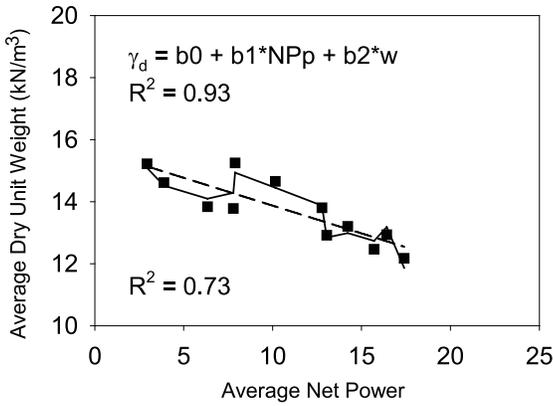
Relationship between dry unit weight and machine power for topsoil
