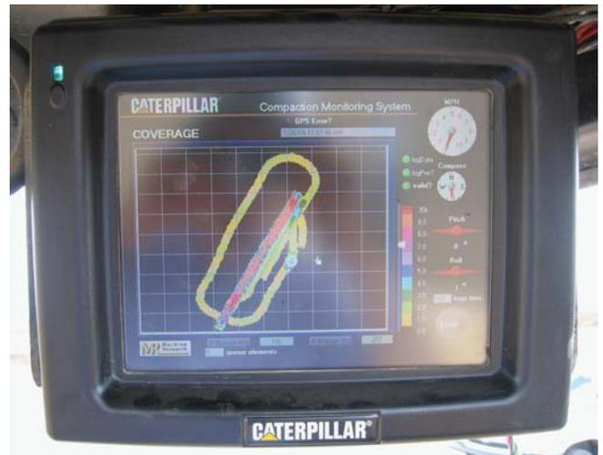
*Number of roller passes presented in real time to machine operator*
