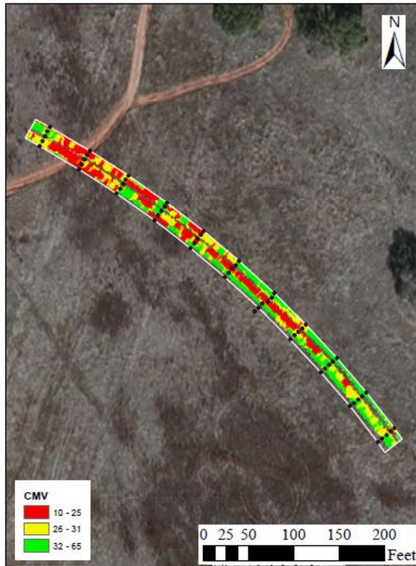
Figure A.6.40. Spatial variation of CMV data from retrofit system on SAKAI roller during compaction of second HMA lift
