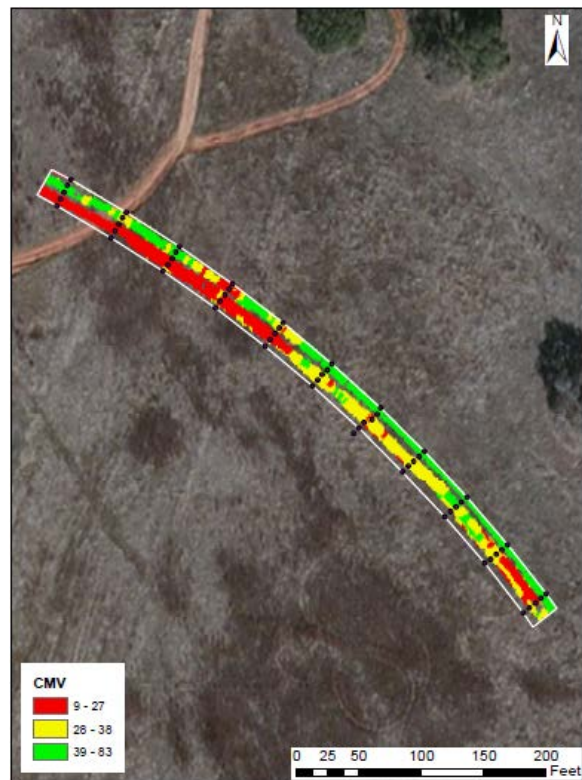
Figure A.6.33. Spatial variation of CMV data from retrofit system on SAKAI during compaction of first HMA lift
