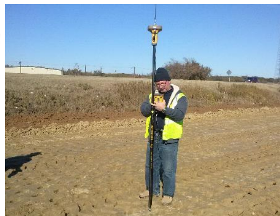
Figure B.1.8. Mapping the test section on compacted soil layer using a local base station
