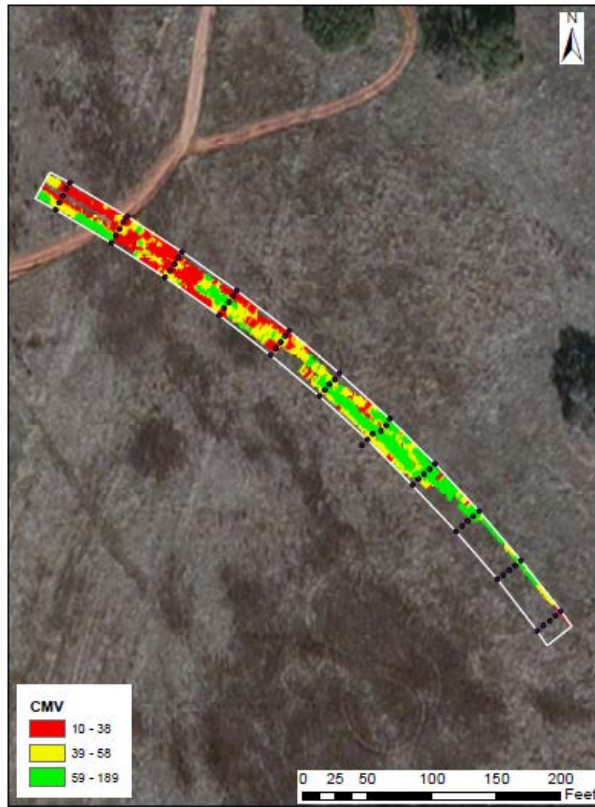
Figure A.6.7. Spatial variation of CMV data from HAMM retrofit system during pre-mapping
