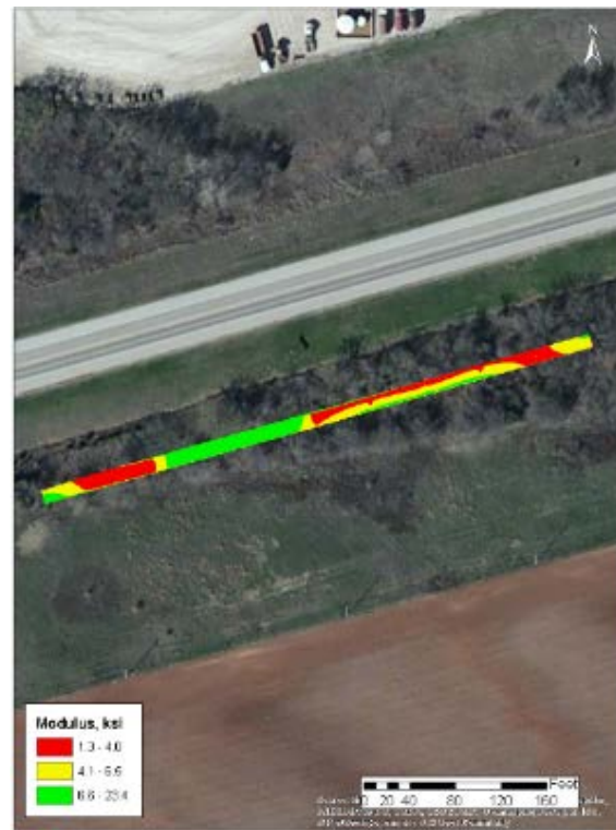
Figure B.3.6. Spatial variation of LWD modulus on embankment layer
