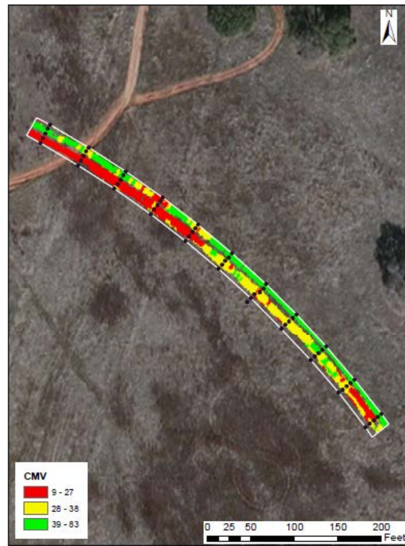
Figure A.6.25. Spatial variation of CMV data from SAKAI retrofit system during compaction of first HMA lift
