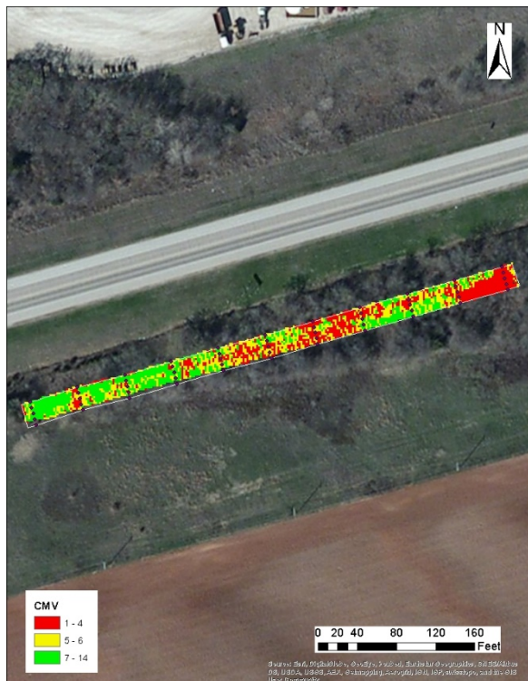
Figure B.4.33. Spatial variation of CMV data from SAKAI retrofit system during mapping of subgrade layer
