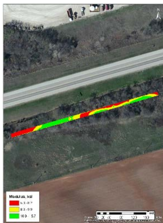
Figure B.3.10. Spatial variation of DCP modulus on subgrade layer
