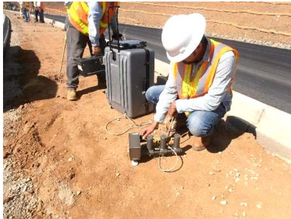
Figure A.1.6. PSPA test
