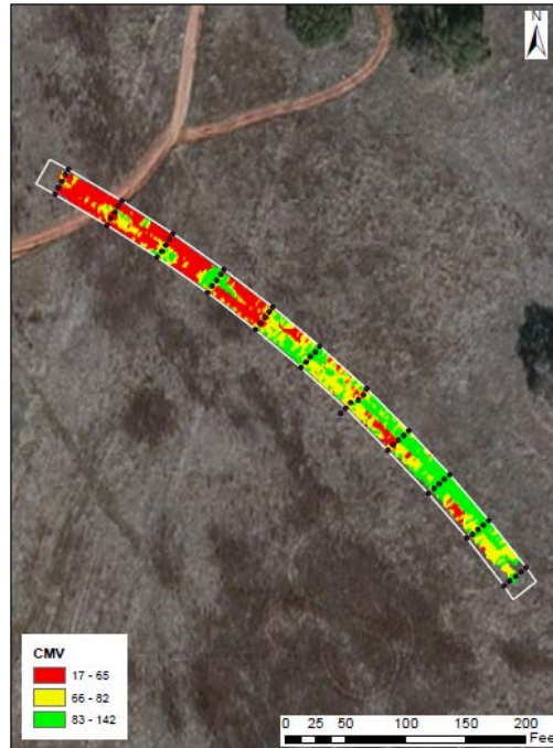
Figure A.6.3. Spatial variation of CMV data from CAT system during pre-mapping
