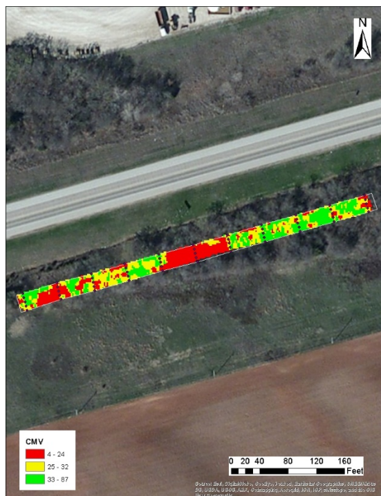
Figure B.4.5. Spatial variation of CMV data from CAT smooth drum roller during pre-mapping (day 2)
