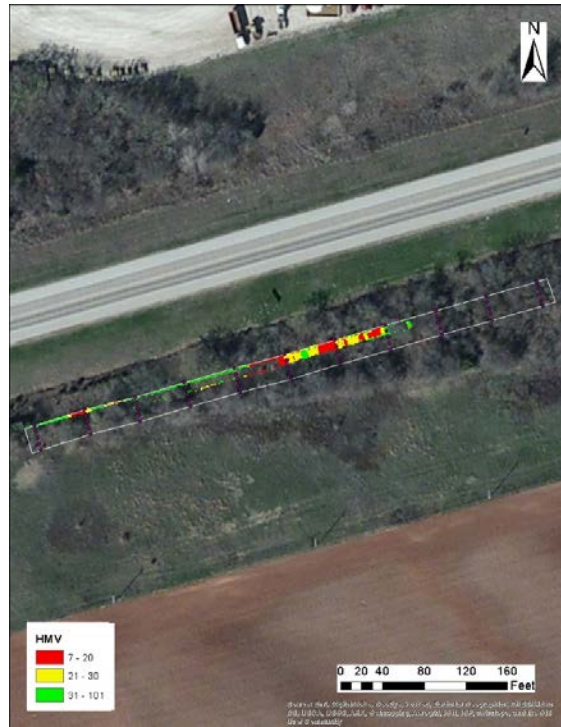
Figure B.4.10. Spatial variation of HMV data from HAMM OEM system during pre-mapping (day 2)
