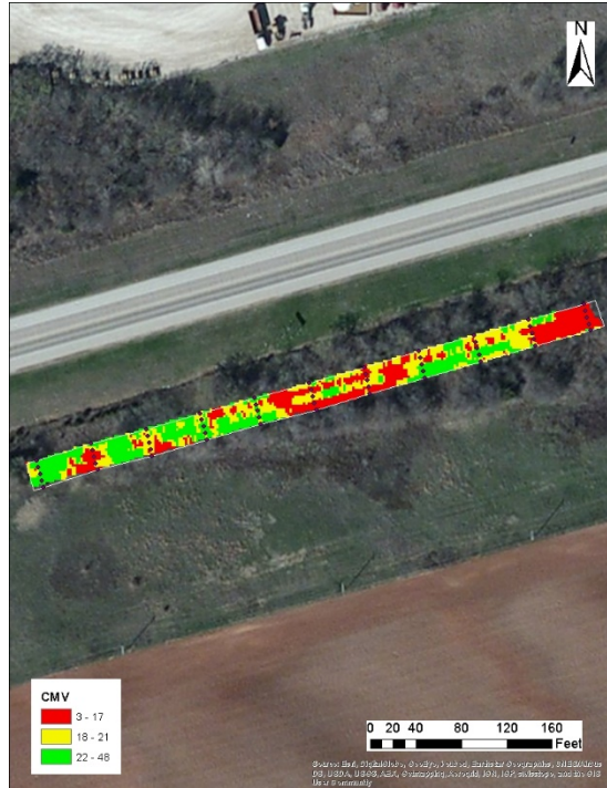
Figure B.4.43. Spatial variation of CMV data from CAT smooth drum roller during mapping of subgrade layer after 18 hrs (day 4)
