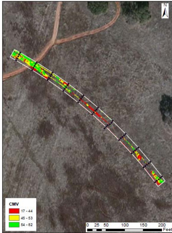
Figure A.6.24. Spatial variation of CMV data from HAMM retrofit system during compaction of first HMA lift
