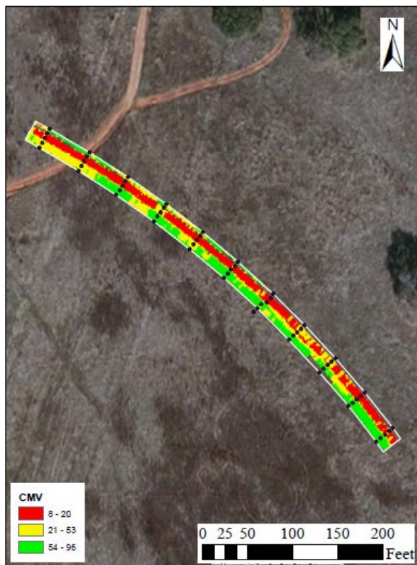
Figure A.6.36. Spatial variation of CMV data from CAT roller during compaction of second HMA lift
