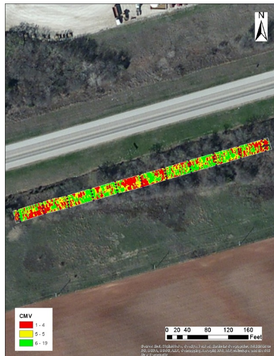
Figure B.4.4. Spatial variation of CMV data from SAKAI Retrofit system during pre-mapping (day 2)
