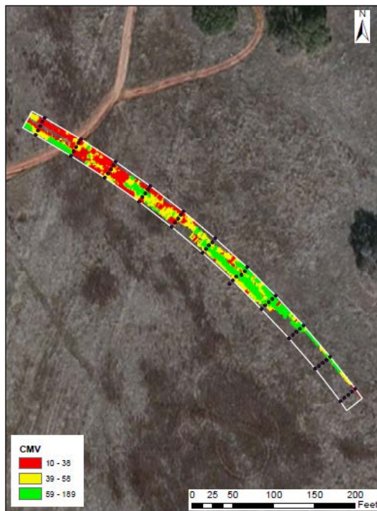
Figure A.6.1. Spatial variation of CMV data from HAMM retrofit system during pre-mapping
