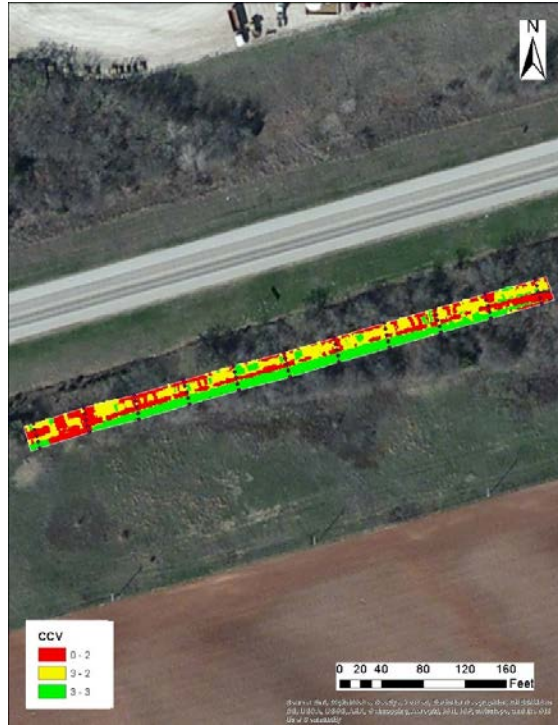
Figure B.4.14. Spatial variation of CCV data from SAKAI OEM system during pre-mapping (day 2)
