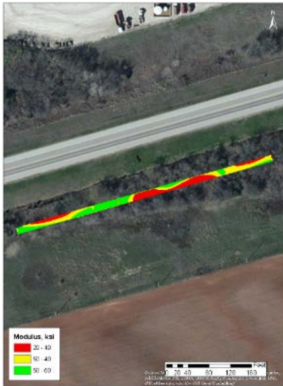
Figure B.3.5. Spatial variation of PSPA modulus on embankment layer
