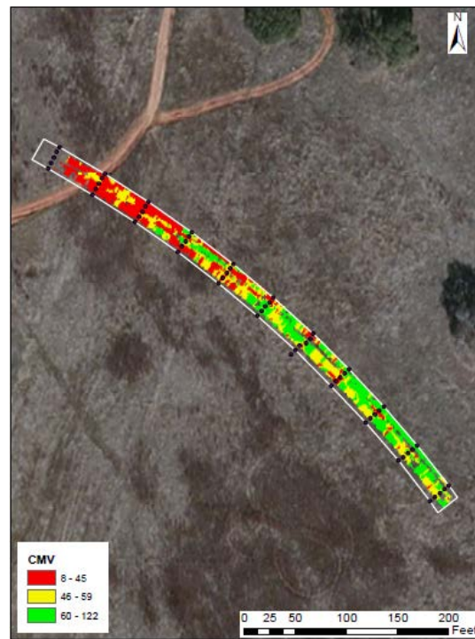
Figure A.6.2. Spatial variation of CMV data from SAKAI retrofit system during pre-mapping
