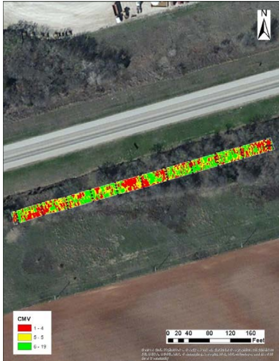
Figure B.4.13. Spatial variation of CMV data from SAKAI retrofit system during pre-mapping (day 2)
