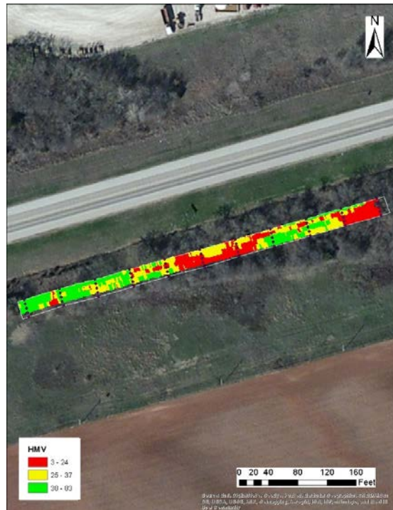
Figure B.4.30. Spatial variation of HMM data from HAMM OEM system during mapping of subgrade layer
