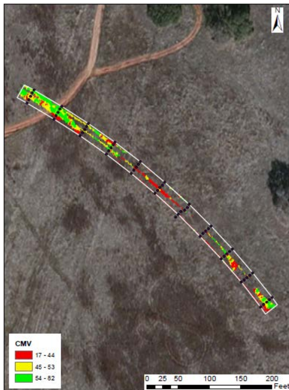
Figure A.6.28. Spatial variation of CMV data from retrofit system on HAMM during compaction of first HMA lift
