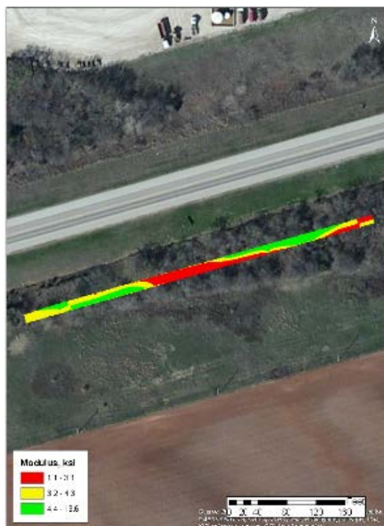
Figure B.3.9. Spatial variation of LWD modulus on subgrade layer
