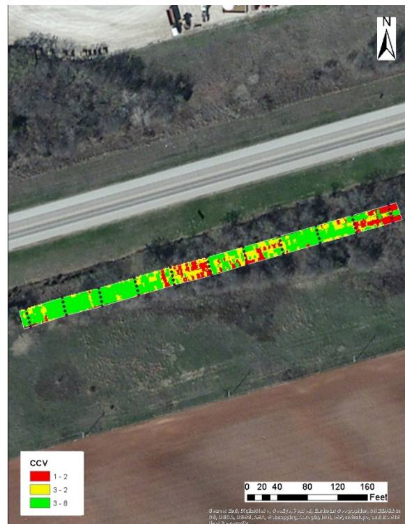
Figure B.4.34. Spatial variation of CCV data from SAKAI OEM system during mapping of subgrade layer
