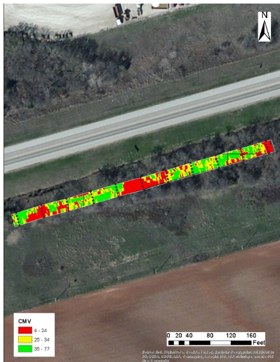
Figure B.4.3. Spatial variation of CMV data from HAMM Retrofit system during pre-mapping (day 2)
