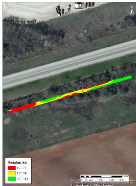
Figure B.3.5. Spatial variation of PSPA modulus on embankment layer
