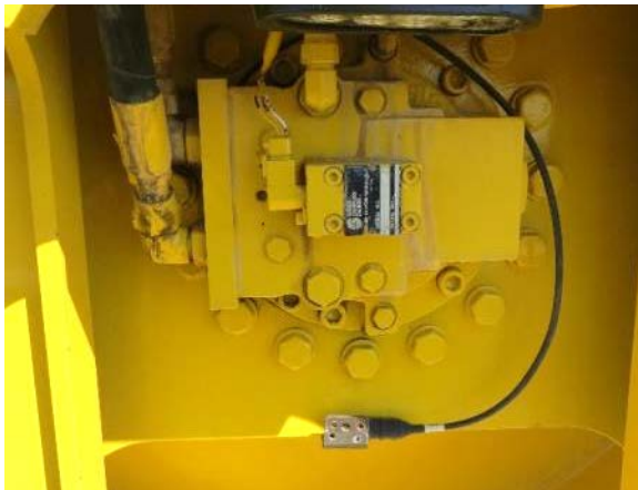
Figure A.5.7. Mounted accelerometer on the roller
