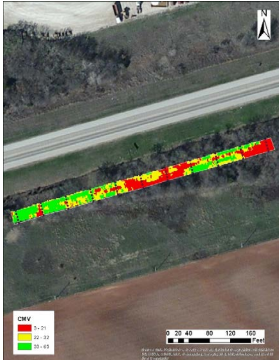
Figure B.4.29. Spatial variation of CMV data from HAMM retrofit system during mapping of subgrade layer
