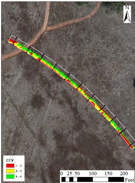
Figure A.6.32. Spatial variation of CCV data from OEM system on SAKAI during compaction of first HMA lift
