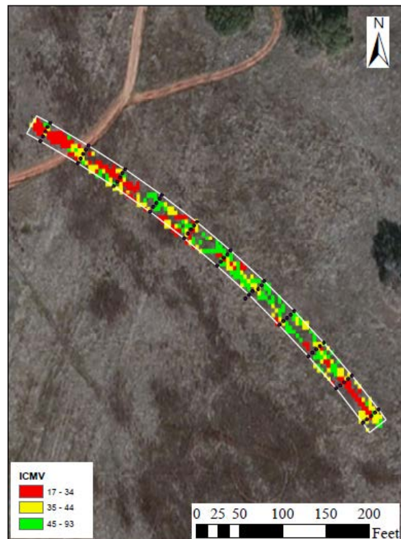
Figure A.6.29. Spatial variation of ICMV data from OEM system on HAMM during compaction of first HMA lift
