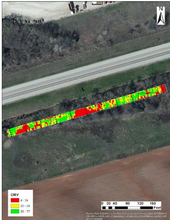
Figure B.4.9. Spatial variation of CMV data from HAMM retrofit system during pre-mapping (day2)
