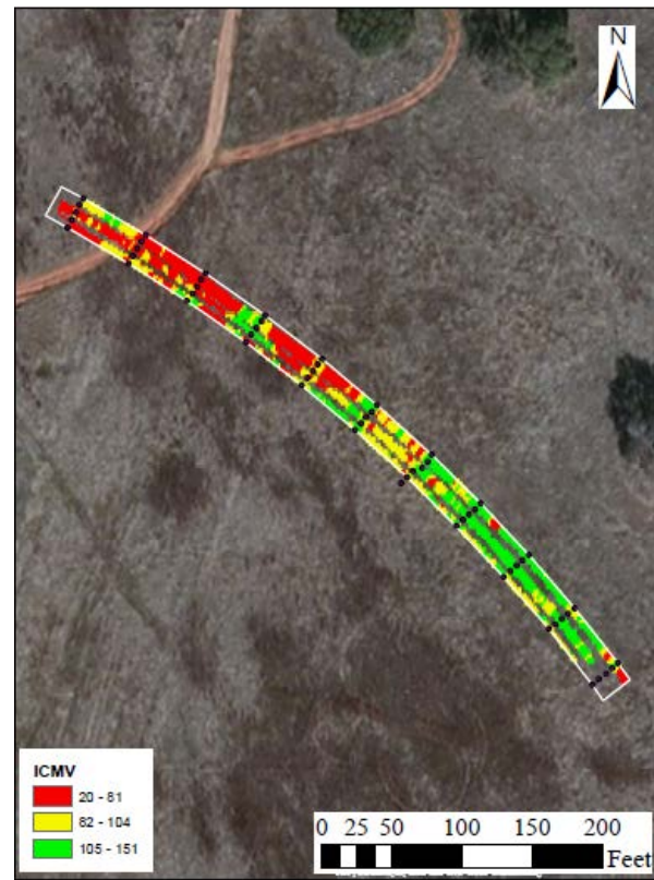
Figure A.6.8. Spatial variation of CMV data from HAMM OEM system during pre-mapping
