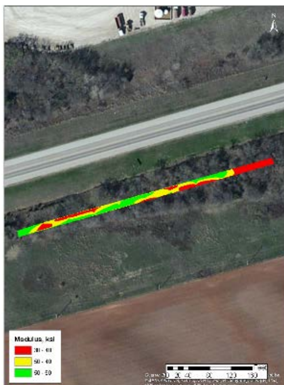
Figure B.3.8. Spatial variation of PSPA modulus on subgrade layer
