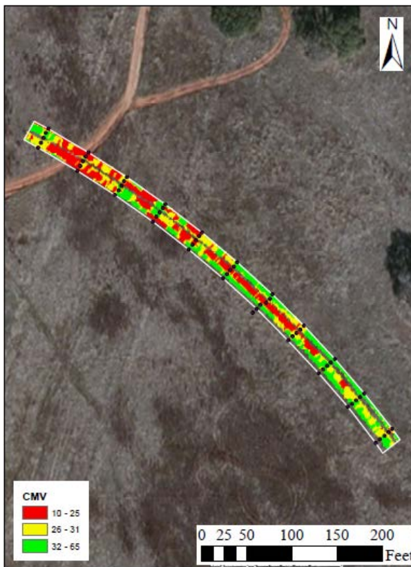
Figure A.6.37. Spatial variation of CMV data from retrofit system on SAKAI during compaction of second HMA lift
