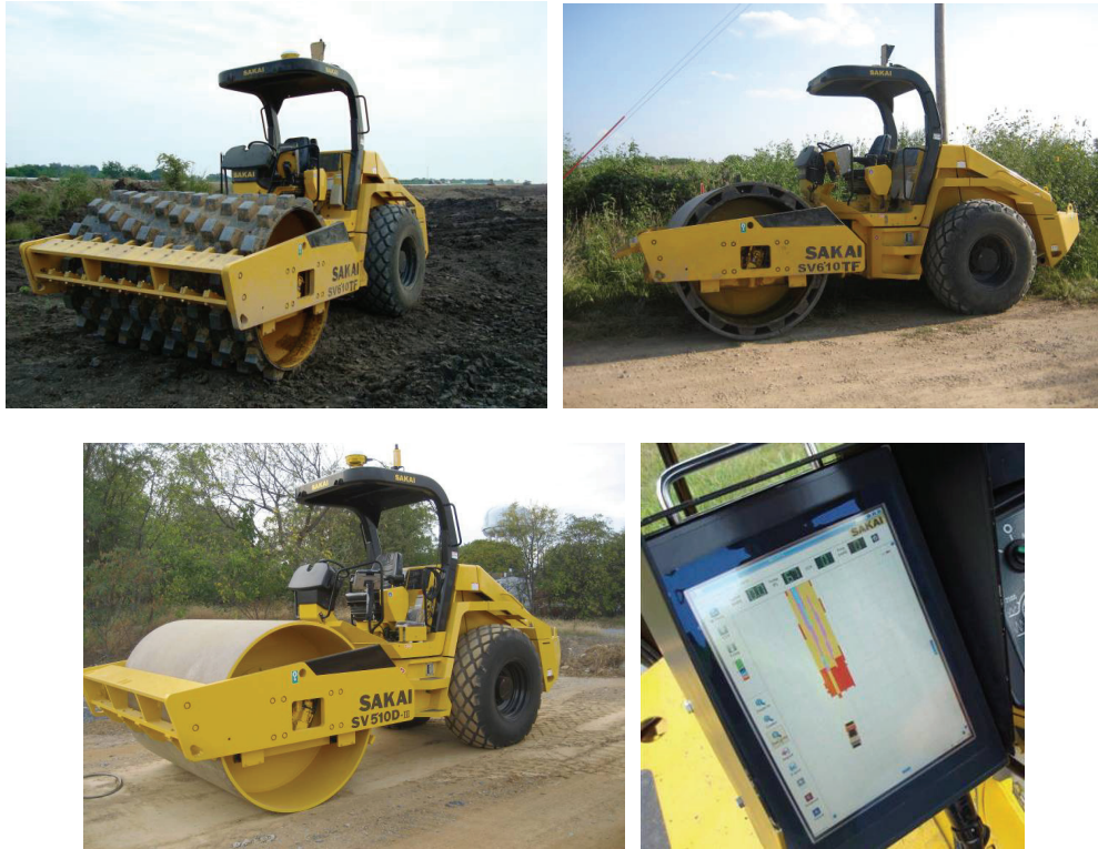
Figure 20. Sakai rollers (padfoot and smooth drum) equipped with roller-integrated CCV measurement system and on-board display unit with Aithon-MT ® software.
