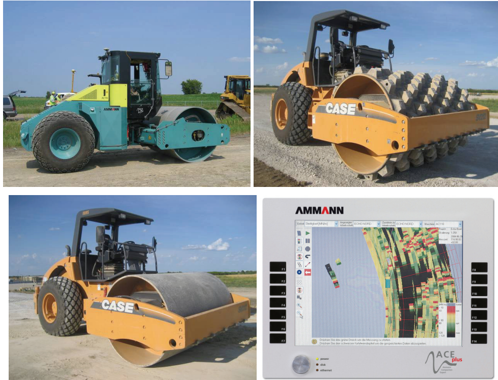
Figure 16. Ammann and Case rollers (padfoot and smooth drum) equipped with roller-integrated k_s measurement system on-board display units with ACE-Plus ® software.
