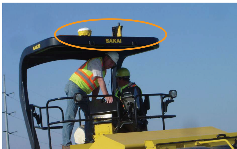
Figure 9. RTK GPS receiver and antenna on a Sakai roller (ICPF MnDOT demo).
