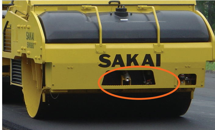
Figure 6. Infra-red temperature sensor on a Sakai IC roller.
