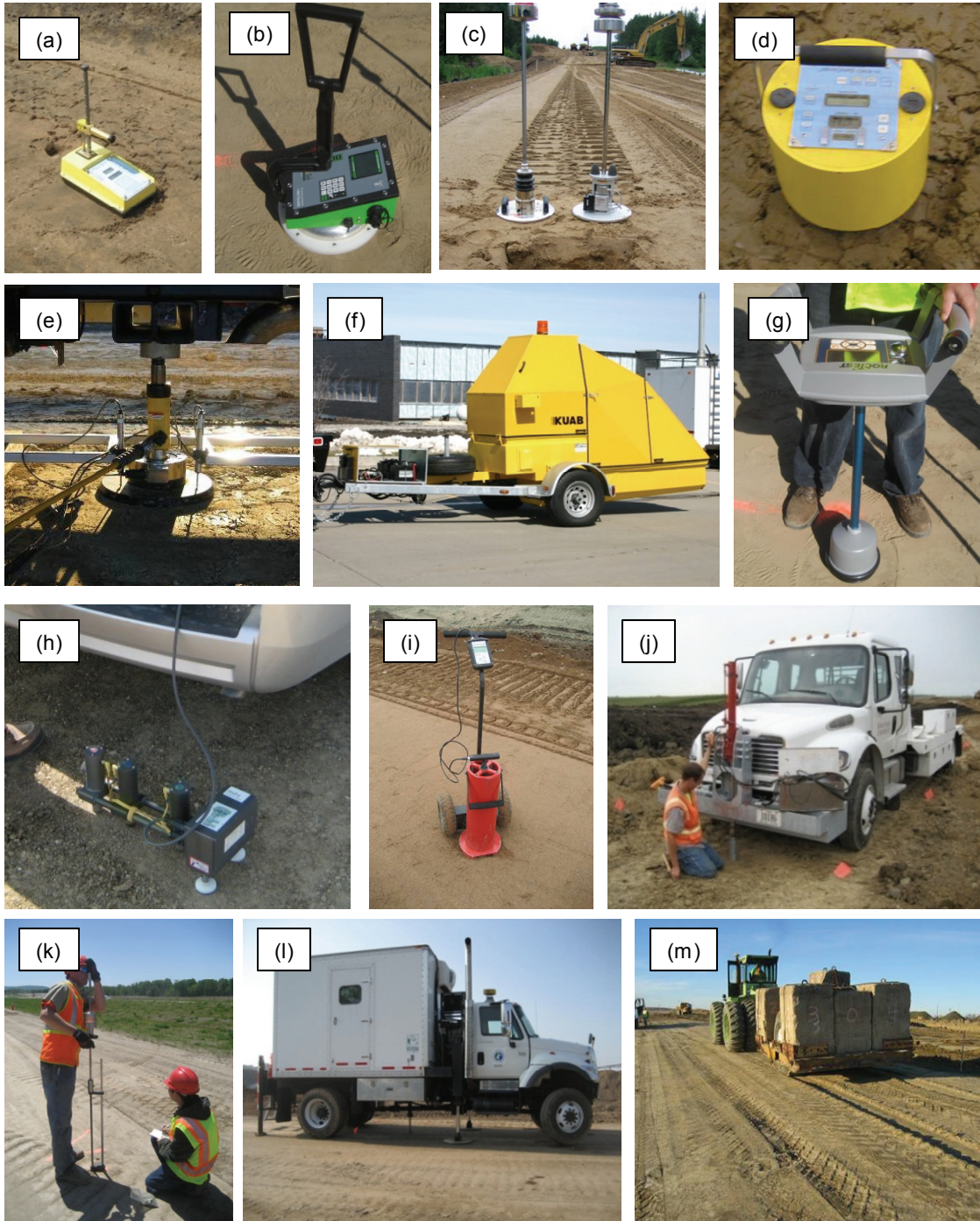
Figure 28. Various in-situ QC/QA test measurements: (a) nuclear moisture-density gauge; (b) electrical density gauge; (c) light weight deflectometers; (d) soil stiffness gauge; (e) static plate load test; (f) falling weight deflectometer; (g) Briaud compaction device; (h) seismic pavement analyzer; (i) Clegg hammer; (j) shelly tube sampling; (k) dynamic cone penetrometer; (l) static cone penetrometer; and (m) heavy test rolling.
