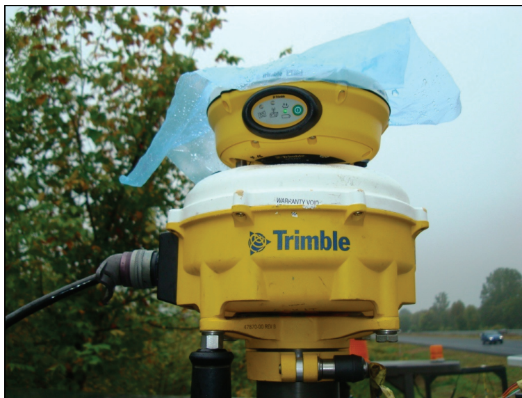
Figure 194. Validation of roller mounted GPS with a hand-held rover (ICPF VADOT demo).
