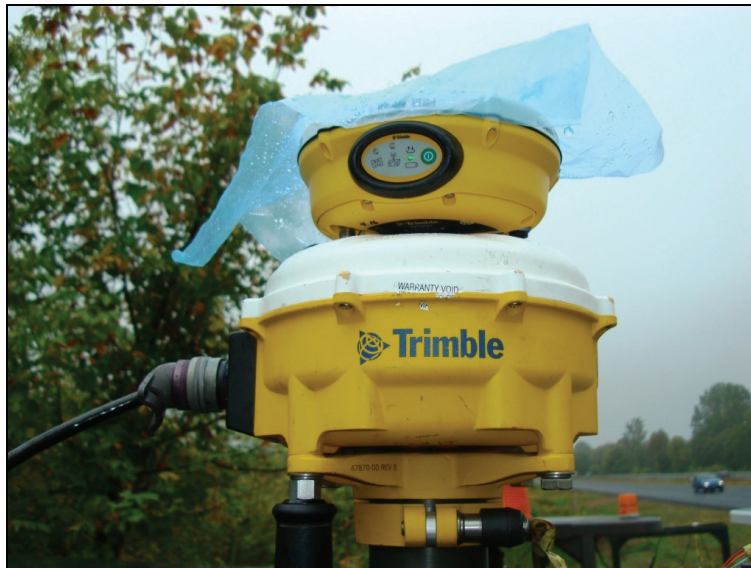
Figure 14. Validation of roller mounted GPS with a hand-held rover.
