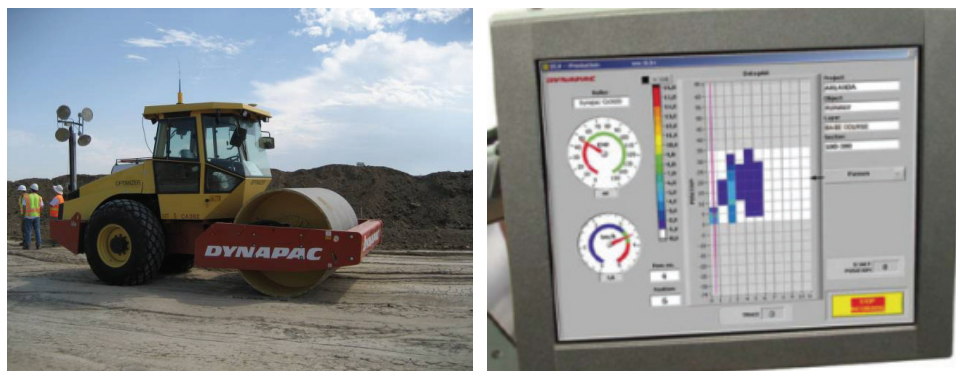
Figure 19. A single-drum Dynapac roller equipped with roller-integrated CMV measurement system and on-board display unit with DCA ® software.
