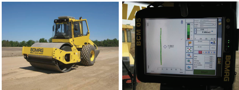
Figure 17. A single-drum Bomag roller equipped with roller-integrated E_{VIB} measurement system on-board display units with BCM-05 ® software.
