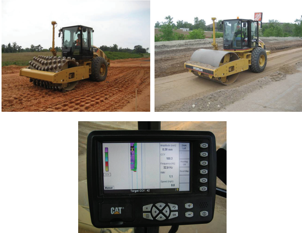
Figure 18. Caterpillar rollers (padfoot and smooth drum) equipped with roller-integrated MDP and CMV measurement systems on-board display unit with AcuGrade ® software.
