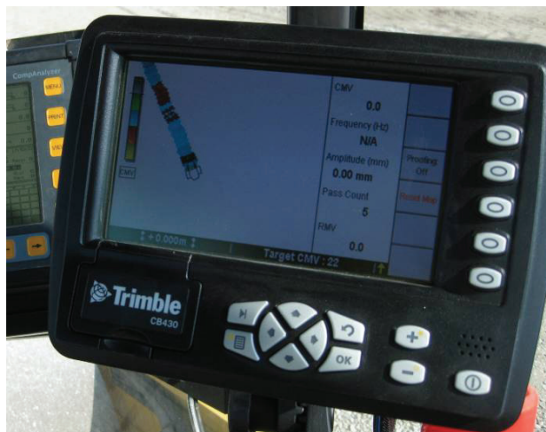
Figure 21. Trimble CB430 on-board display unit with roller-integrated CMV measurement system.
