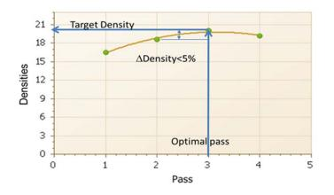
Linear regression relationships between the point test results and the IC-MV results will be used to establish the production target IC-MV that meets the in-place compaction requirements of P-401. A linear regression curve example is as follows.
