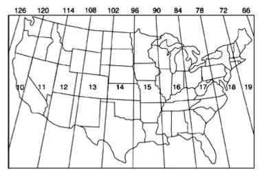
2. Provide Base Station(s) as ground mounted or virtual GPS base units that record values in northing, easting, and the elevation data in meters using the UTM coordinate system along with the longitude/latitude of the measurement values. Ensure the GPS base station broadcasts updated correction data to the GPS receivers on the IC rollers and the hand-held rovers during operations with a survey tolerance of not greater than 1.6 in. (40 mm) in both the horizontal (x and y) directions.
