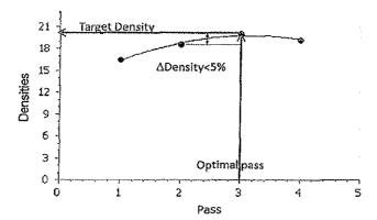
Linear regression relationships between the point test results and the IC-MV results will be used to establish the production target IC-MV as the target density (% G<sub>mm</sub>) meets the MassDOT inplace compaction requirements. A linear regression curve example is as follows.
