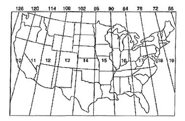
The State Plane Coordinate system can be used and set as North American Datum of 1983 (NAD83) for this project. Ad-hoc local coordinate systems will not be allowed.
