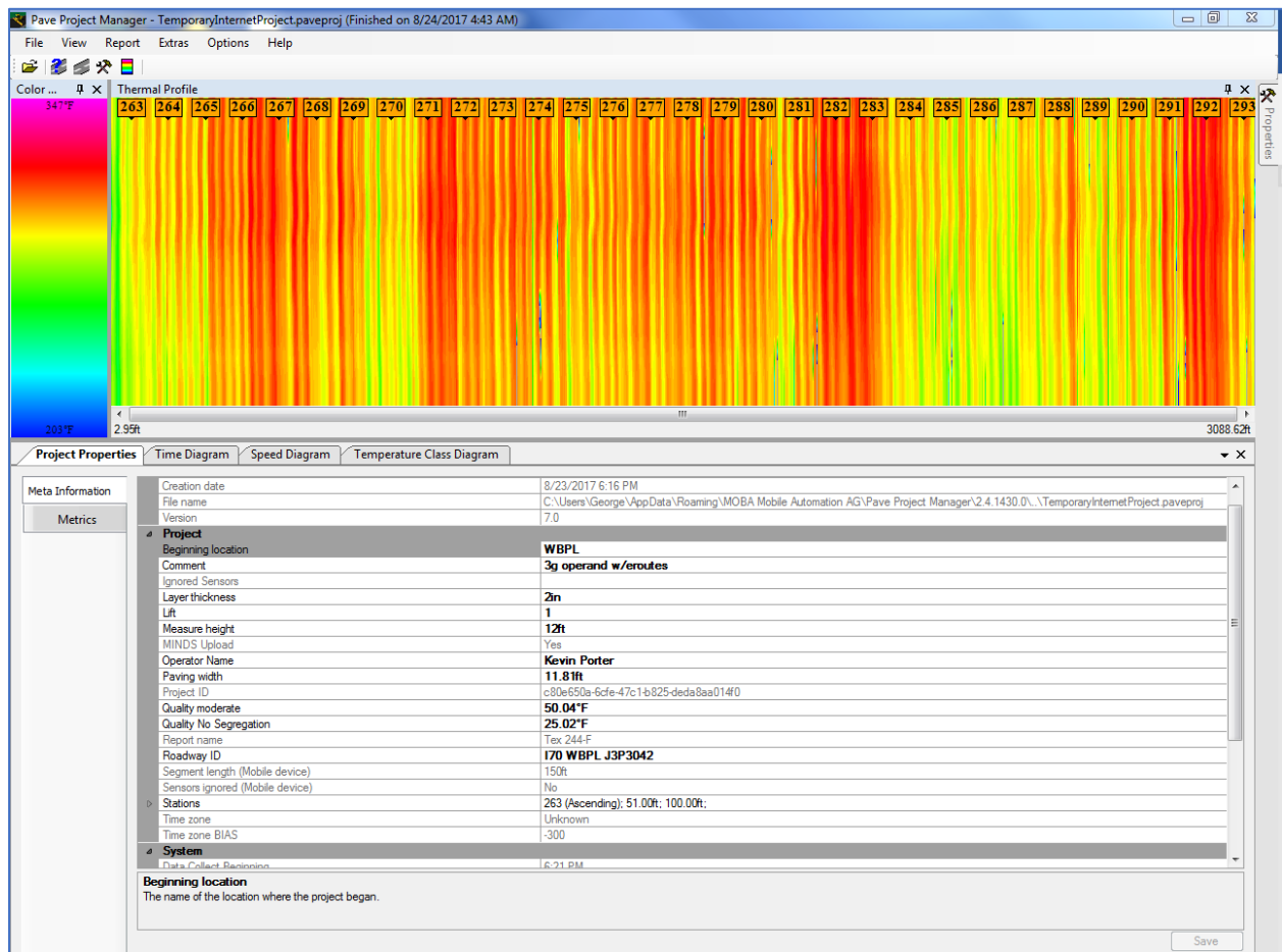
Figure 60: Incorrect distance reported by MOBA PPM for the data on 8/23/2017 (J3I3042, I-70).
