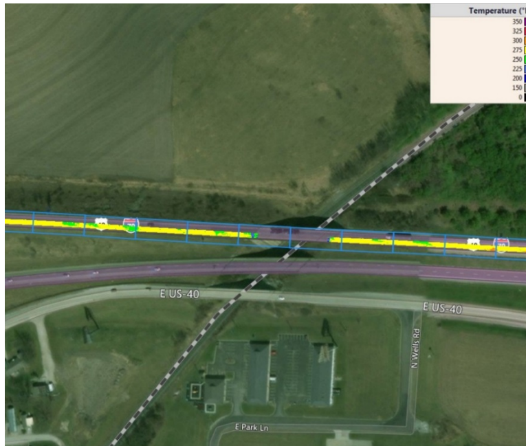
Figure 28: Example of a Veta Sublot screen for IR data analysis (J3I3042, RT70).
