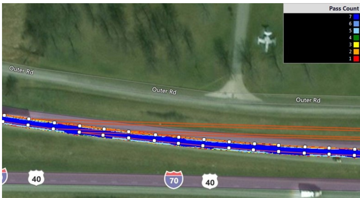
Figure 65: Incorrect Boundary File for 8/23/2017 (Project No. 3 - J3I3042, I-70).
