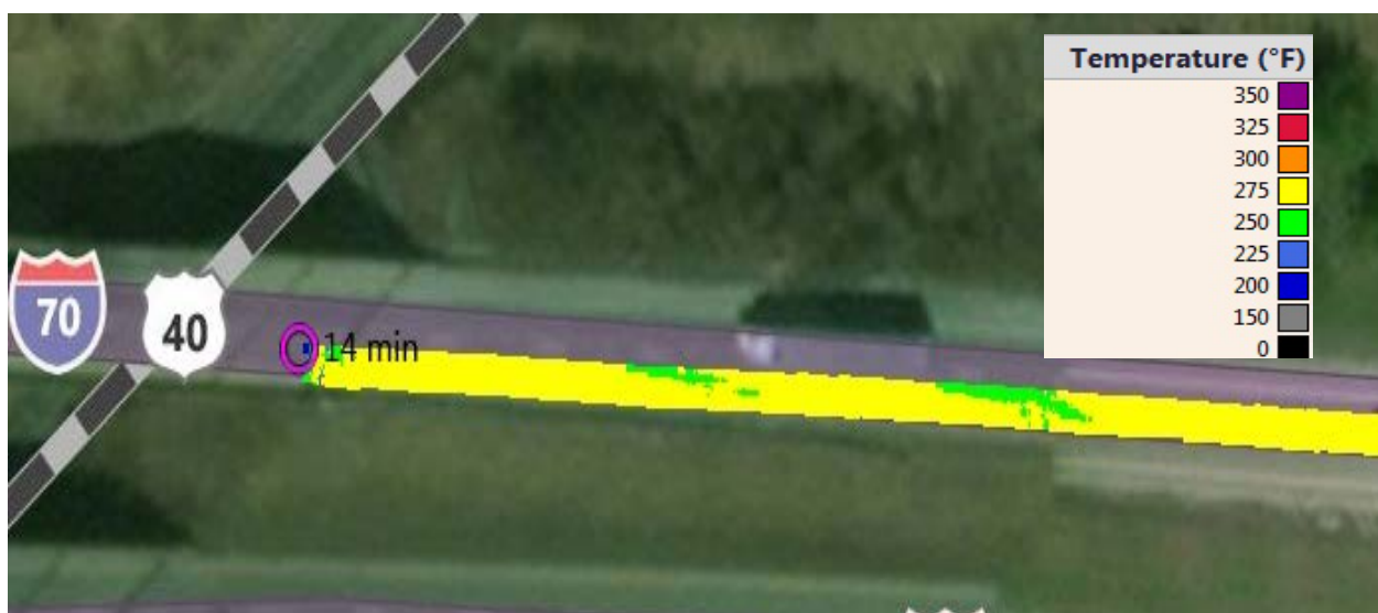
Figure 31: Example of a Veta Paver Stop plot (J3I3042, RT70).
