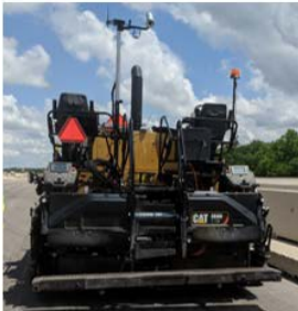
Figure 4. Trimble/Caterpillar thermal imaging system
