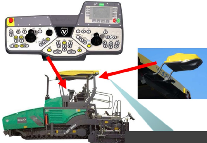
Figure 1. Vogele RoadScan thermal imaging system
