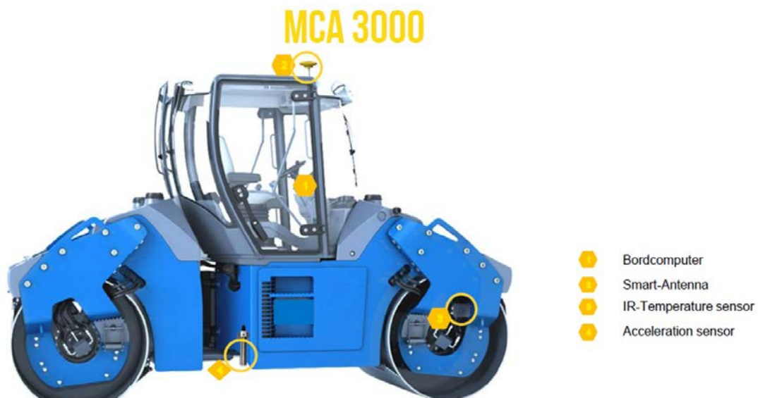
Figure 6. MOBA MCA (MOBA Compaction Assist)
