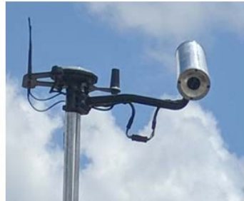
Figure 4. Trimble/Caterpillar thermal imaging system
