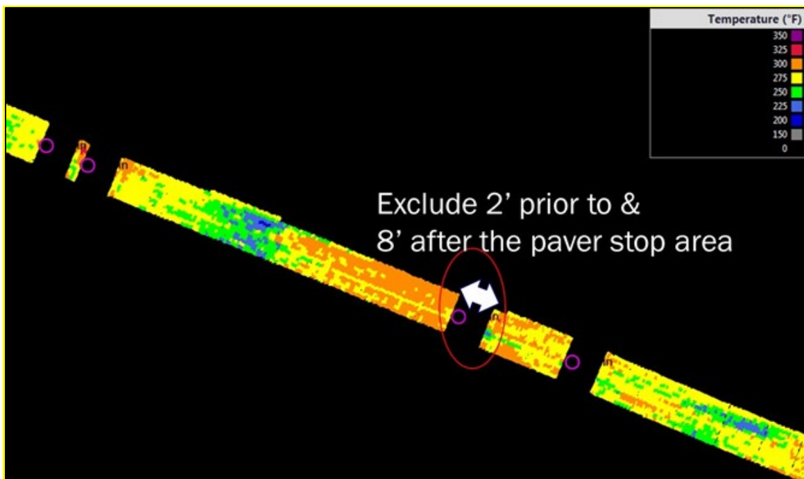
Figure 18: AASHTO PP80 IR Analysis Method: 10' Exclusion Around a Paver Stop Location.
