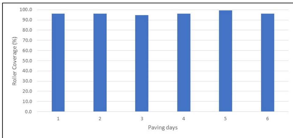
Figure 97: Summary of Roller Coverage Report for J7S3117, LP49.
