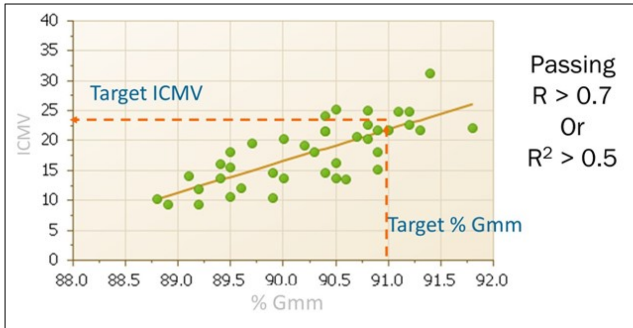
Figure 33: Target ICMV Determined by Correlation Between ICMV and Acceptance Spot Tests from Trial Section Data.
