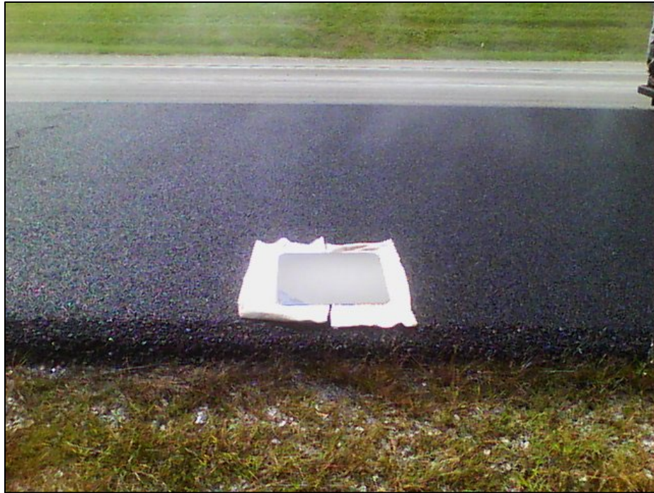
Figure 24. Photo. Improvised reference object met the dimensions required and stayed below 150°F during testing.
